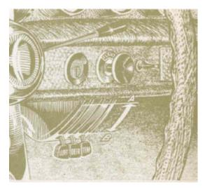
When the "Temp" control is altered, there will be a slight delay before the thermostat in the heater has stabilised itself at the desired temperature. In very cold weather, particularly if the car is full of passengers, there can be misting on the windows. The best way to get rid of this or to avoid it is to have the ventilator window fully or partially open at the same time as the fan motor is running at full output and the defroster control in its fully open position.
